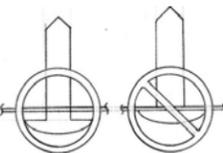
**NOTE:** to ensure a proper water tight seal put a bead of silicone caulk into the Wall Trim only where the cut edge of the Panel is inserted. ( Figure 12).
